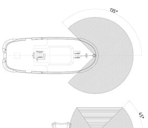
operations, with the towing line at an angle which can reach up to 135 degrees from centre line and 45 degrees from horizontal. This ideally suits the modern very manoeuvrable and powerful escort and harbour tugs.
